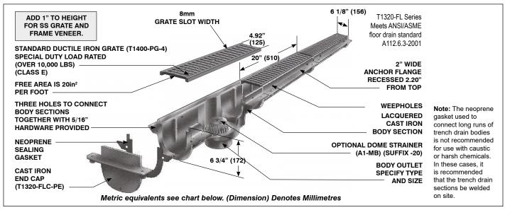
**Note:** Specify total length of trench drain required in 20" long sections. Section "A" is standard with a bottom outlet (specify bottom outlet connection type and number and location of outlets required). Section "B" does not have a bottom outlet. Any number of Sections "A" and "B" can be bolted together to produce any length required.
