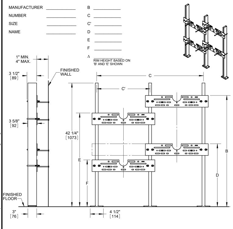
RECOMMEND ALL FEET BE SECURED TO FLOOR WITH 1/2" BOLTS AND ANCHORS BY OTHERS
