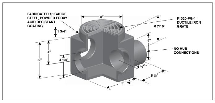
Note: The function of the BV1290 is to provide a sump with multiple inlets that the foundation drain lines connect to.
