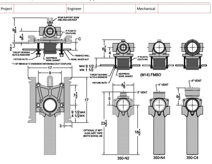
**Regularly Furnished:** Vertical water closet carrier with floor mounted foot support, rear anchor, 7"ABS coupling, rear anchor support, & faceplate.
