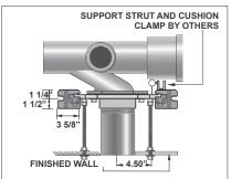
**Note:** 8" tapered thread ABS nipple shipped standard with MC-10 Series carriers. The universal faceplate assembly accepts all nipple variations, rolling thread (-OR), cast iron (-CI) and tapered thread ABS with adjustable horn (-AH).
