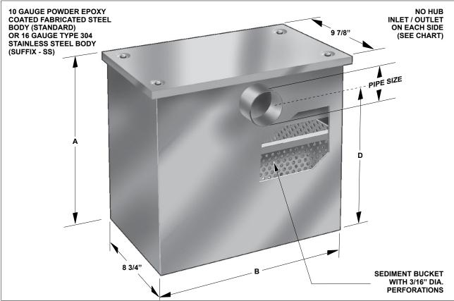
Note: Minimum of 12" (depending on the Model selected) is required above the lid for easy removal of the sediment bucket.
