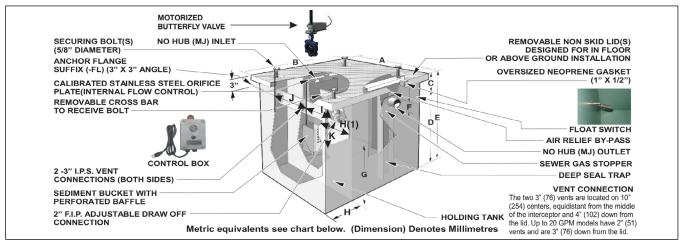
Note: The "C" dimension detailed above is from either the middle of the inlet or the outlet to the top the interceptor. The inlet and outlet dimensions are always the same.
