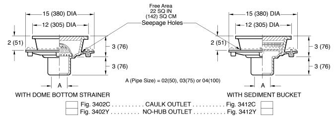
NOTE: When NO-HUB outlet is specified a caulk outlet w/9502 Speedi-Seal gasket will be supplied
