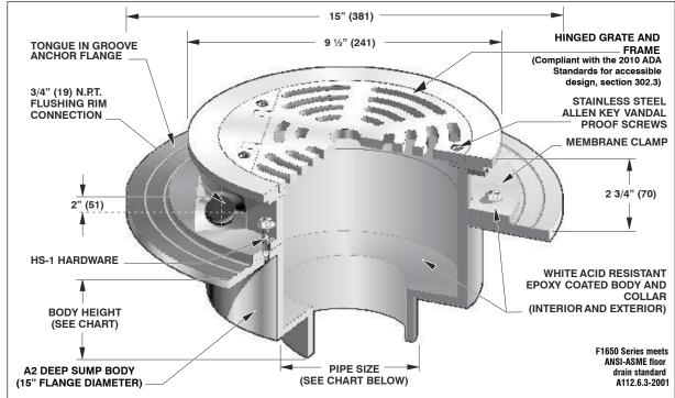
**Note:** See F1670 for water supply control box to be used with the flushing rim floor drain Use a vacuum breaker between the potable water supply and the connection to the flushing rim connection (by others).
