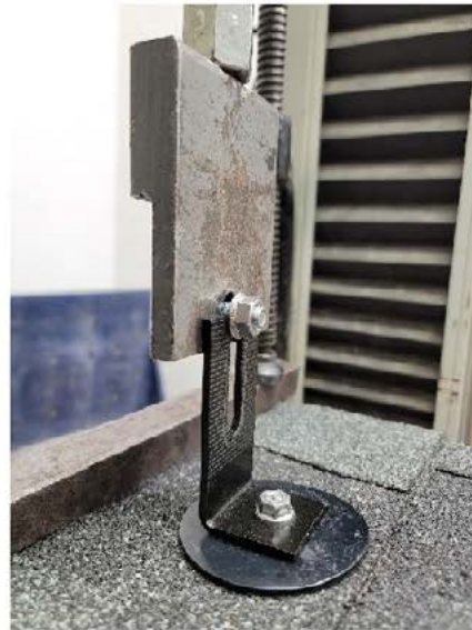
Figure 1b. Typical failure mode.
