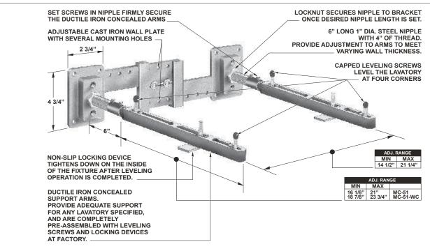
MC-51 Series Meets ANSI/ASME fixture carrier standard A112.6.1M-97
