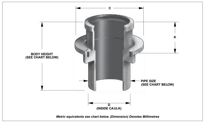
**Note:** The R1854 is made out of lacquered cast iron material. All other sizes are made from fabricated 14 gauge galvanized steel that is powder, epoxy coated with an electro-static application. These models are standard with an acid resistant epoxy finish.
