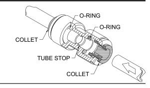
Pull on the fitted tubing to ensure it is secure.
