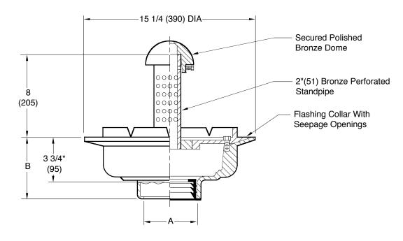
Fig. 2685C . . . CAULK OUTLET Fig. 2685Y . . . NO-HUB OUTLET
