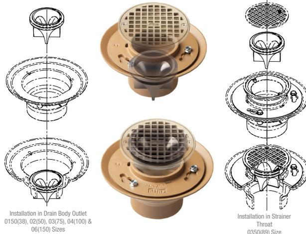
**INSTALLATION:** The 0150(38), 02(50), 03(75), 04(100) & 06(150) Quad Close Trap Seal sizes install in the drain outlet. The 0350(89) Quad Close Trap Seal size installs in the throat of adjustable strainers. To install simply insert the Quad Close Trap Seal in the drain outlet or throat of strainer until the top of it is flush with top of drain outlet or strainer throat.
