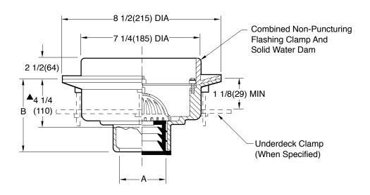
Fig. 3960C ..... CAULK OUTLET Fig. 3960Y.....NO-HUB OUTLET Fig. 3960T ..... THREADED OUTLET
