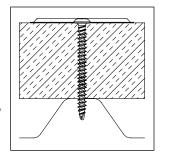
Head: #3 Phillips Head Height: .118" max Head Dia: .448" max Thread Major Dia: .238" Shank Dia: .180" Strength (lbs ult.): Tensile: 3600 Torsional: 110 in-lbs min Shear: 2630 Pull-out: (lbs avg.): 22 ga: 540 20 ga: 630 18 ga: 900 4000 psi concrete (1" penetration): 850 3/4" plywood (through penetration): 590 2x dimensional lumber (1" penetration): 605
