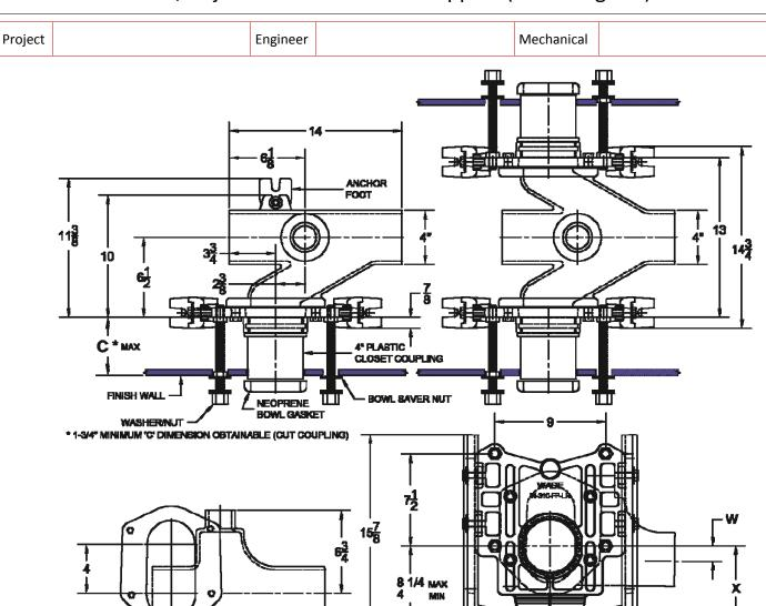
Connection Orientation Model Type 311LR-NL3 Left 311LR-NR3 Right 311LR-ND3 Double No-Hub 311LR-NL4 Left 311LR-NR4 Right 311LR-ND4 Double
