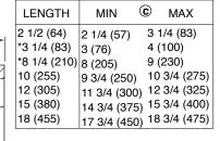
NOTE: When nipple lengths between 3 1/4" (83) and 8 1/4" (210) are specified, the 8 1/4" (210) nipple will be supplied. Nipple must be cut to specified length by
