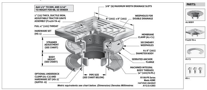
Note: When used as a floor or area drain in exterior areas and subject to rainfall, ensure that the free area is equal to twice the transverse (cross sectional) area of the connecting pipe.
