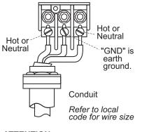
ATTENTION: Unit must be hard wired. NOTE: Heaters are single phase. All tests are measured at the output of the heater.
