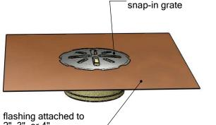
flashing attached to 2", 3", or 4" – bronze no-hub fitting
