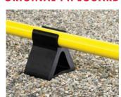
The line of original PipeGuard Pipe Supports is designed to support most common roof-top pipes from ½- to 5-inches in diameter. Made from heavy duty EPDM, PipeGuard does not require any tools for installation. Simply compress base to "open" pipe clamp, and place it around the pipe. Position in place and you're finished. Typical installation time is less than 10 seconds.
