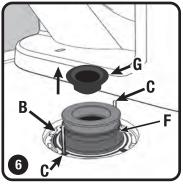
Align toilet over bolts (C) and press toilet firmly onto floor. The wax inside the product will adhere to the floor flange (B). Note: Toilet can be repositioned on seal, if needed, unlike with traditional wax rings. If the toilet doesn't sit flush on the floor, remove the black round plastic insert (G) from inside the Perfect Seal® (F) and reset.
