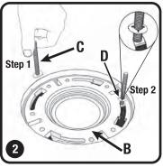
Step 1: Insert bolts (C) into flange (B). Step 2: To stabalize bolts, place plastic washers (D) to base of bolts.
