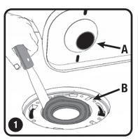
Clean toilet horn (A) and floor flange (B) of all wax residue.
