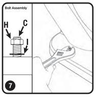
Place metal washers (I) over bolts (C) and tighten nuts (H) (careful not to overtighten). Trim toilet bolts flush to the top of bolt. Cover with toilet bolt caps. Do not overtighten: Bowl or closet flange may crack.
