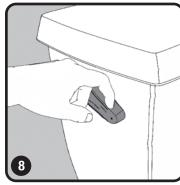
Install supply line and turn on water. Flush toilet and inspect for leaks.
