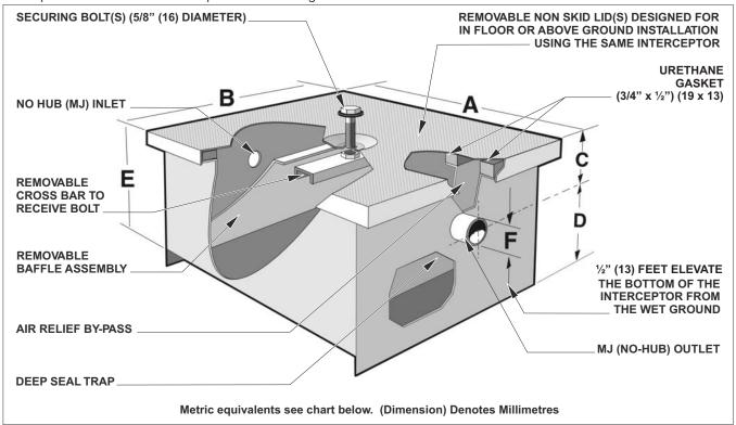
Note: The "C" dimension detailed above is from either the middle of the inlet or the outlet to the top the interceptor. The inlet and outlet dimensions are always the same.
