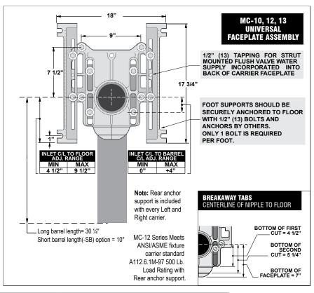
Note: 8" tapered thread ABS nipple shipped standard with MC-12 Series carriers. The universal faceplate assembly accepts all nipple variations, rolling thread (-OR), cast iron (-CI) and tapered thread ABS with adjustable horn (-AH).
