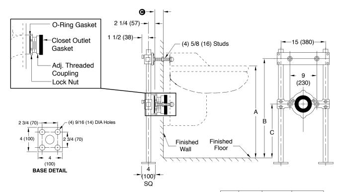
Fig. 0913...... 3" (80) OUTLET CONNECTION Fig. 0914..... 4" (100) OUTLET CONNECTION
