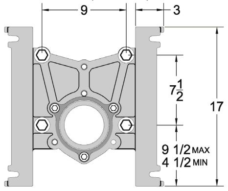
**Regularly Furnished:** Cast iron closet carrier face plate with adjustable feet, 4" NPT waste connection adapter, ABS coupling, neoprene bowl gasket, chrome plated cap nuts and zinc plated hardware. Base must be securely anchored to concrete floor with 1/2" anchors (furnished by others) Rod support feet are provided and must be anchored to floor. Maximum 'C' Dimension is 6" with standard hardware. Longer couplings available when specified.
